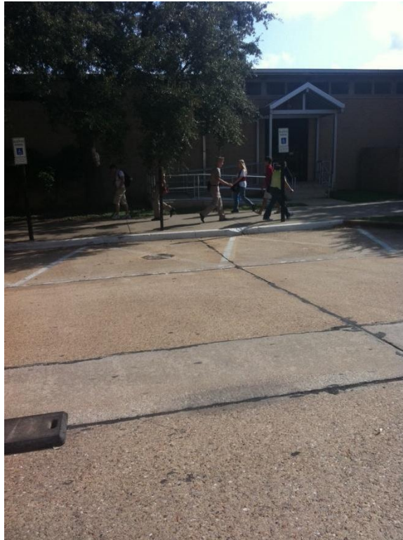
Parking Area Ireland Street - No Compliant Curb Ramp and No Accessible Aisles
