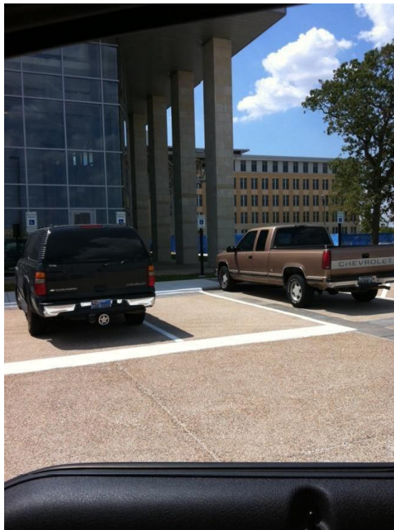
Parking Area 96 - No Compliant Curb Ramp and No Accessible Aisle
